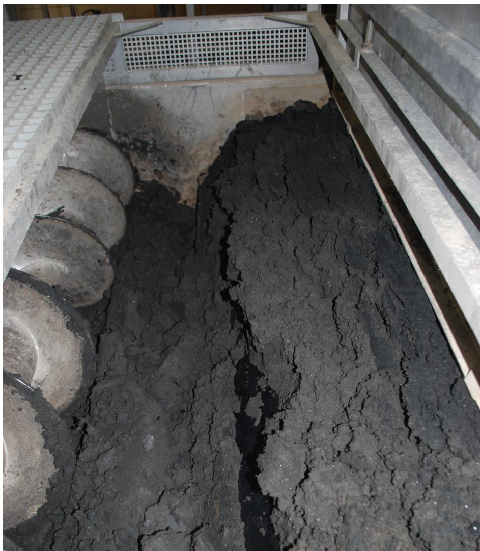
Organic matter-rich struvite from process water from potato processor Aviko Steenderen (The Netherlands) treated in wastewater treatment plant Waterstromen Olburgen. Different water treatment processes yield different forms struvite, ranging from crystals with few impurities to organic matter-rich struvite. The water treatment process determines which struvite is harvested and which applications of this material are possible.
